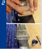
Work in using FinishCork (cork or felt side).
