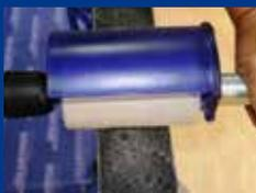
Syntec Race Alpin may then be worked in using the SpeedBrush Fleece with max. 1200 rpm, applying gentle pressure.
