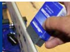
**7** Use the OvalBrush Steel to brush off wax residues from the structure.
