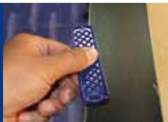
When the edge shows rigidification, pretreat using the DiamondFile Coarse ...
