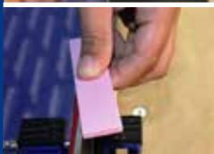
...using the aluminium oxide stone.
