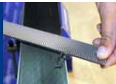
Once the wax has cooled, remove excess FX-Strip material using the CrossFile...
