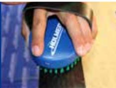
In order to reveal the ski microstructure, brush the base 2 – 3 times in running direction using the OvalBrush Steel MicroFinish.
