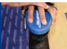
Use the OvalBrush Steel to brush off wax residues from the structure.
