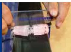
Allow the ski / board to cool for at least 1 to 2 hours. Then scrape the wax from tip to tail using a sharp scraping blade and applying gentle pressure.
