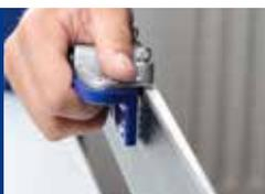
**4** Clamp the RacingFile into the tool (e.g., SteelEdge WorldCup) and grind the side edges to the required relief angle.
