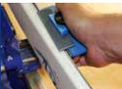
Clamp a CrossFile Mini into the edge grinder and pregrind to the desired angle. Then continue using the RacingFile (Maxi or Mini).
