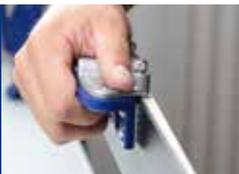
In order to grind the edges precisely, remove any side wall projection using the SideWall Planer Pro.
